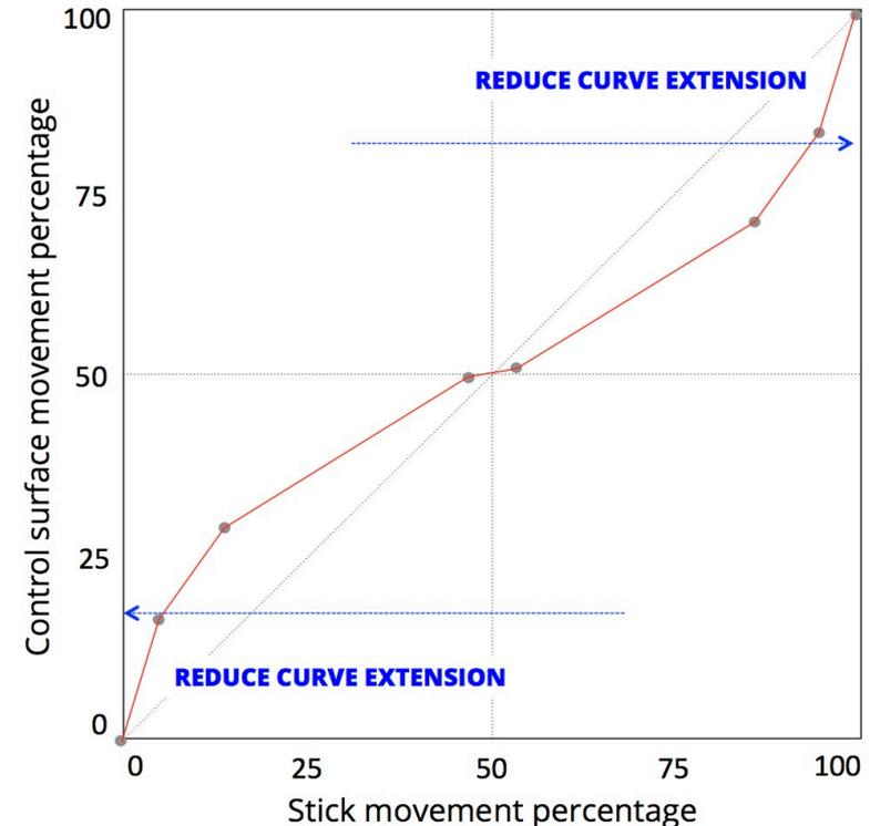
To better control your snaps, regulate the full excursion of aileron, elevator and rudder in presence of different throttle regimes.
