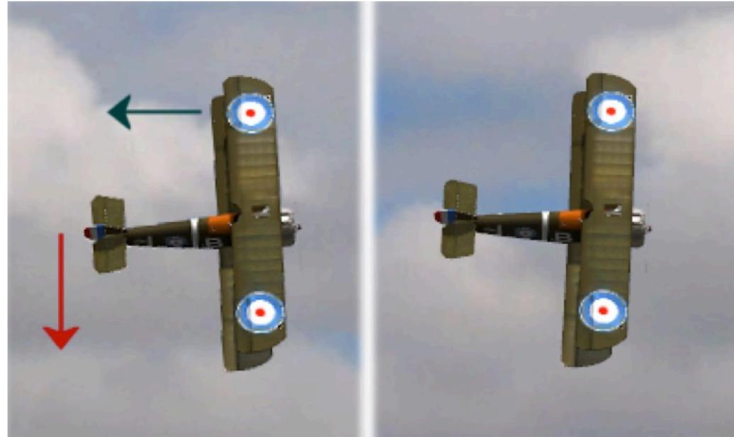
Adverse yaw occurs because a downward deflected aileron causes more drag than the upward deflected aileron. This drag force drifts the airplane out of its flight path during rolls sequences, in a direction opposite to the rolling versus
