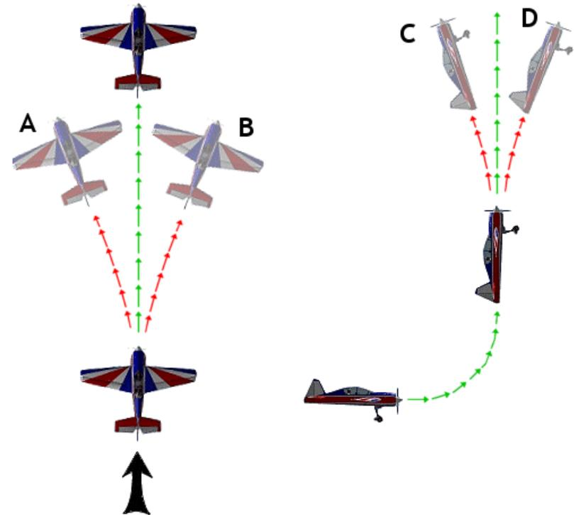
A moderate right yaw and down pitch should be expected and accepted. If their fix would require more than 5 pixel in trim change, as discussed later, than adjust engine incidence versus opposite side.
