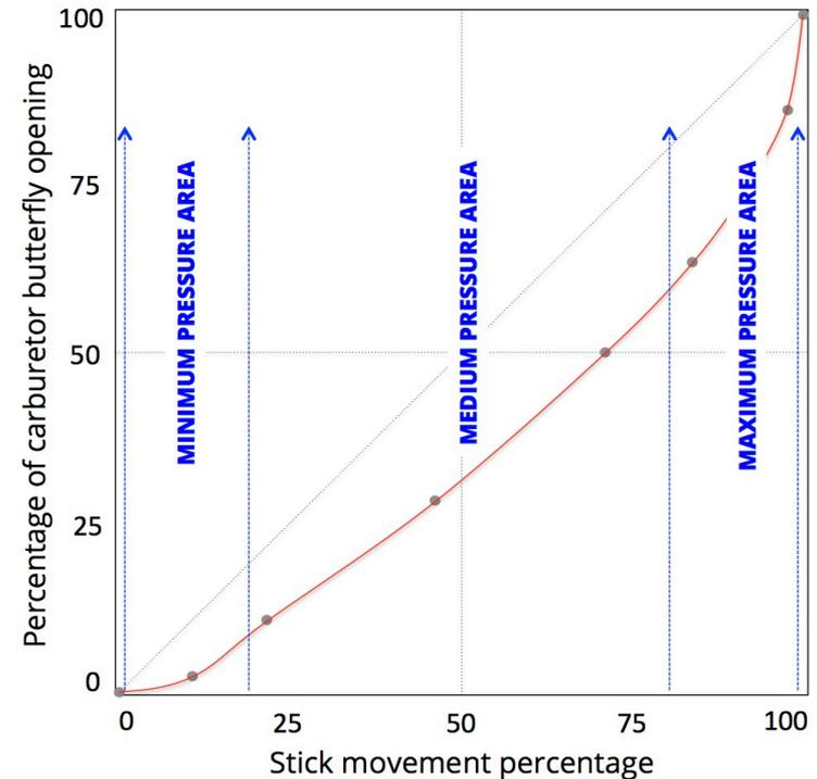
Determine three switch activation areas by setting the stick movement position that will activate the switch
