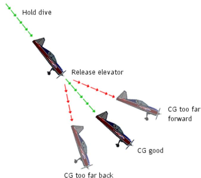
The outcome of these tests is determined by the trimming you introduced at step 1. in order to keep level light. The need for this trimming is significantly determined by the position of the aircraft's CG.
